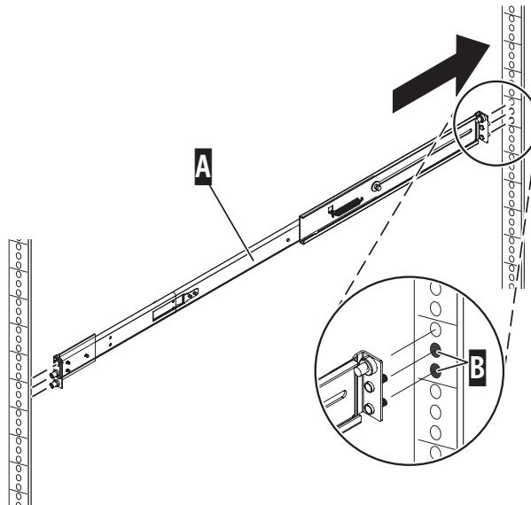
**7.4** Press on the end of the slide rail **A** to compress the spring-loaded mechanism, and insert the slide rail into the front-right rack mounting flange **B** holes.
